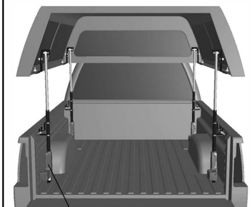
Control Box Goes Here on standard installs
