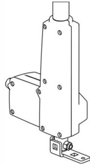
**\*NOTE: Use self-tappers first to ensure bolt will be accessible under truck before drilling hole for 1/4" Carriage Bolt.**
